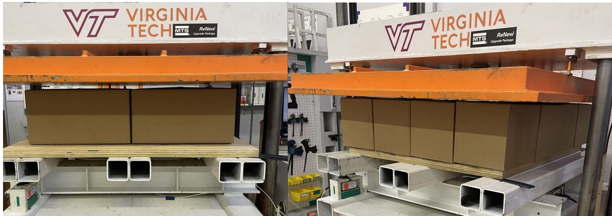
Figure 4. Experimental setup for the box layer compression test. Left: No overhang. Right: 1 in. overhang.
