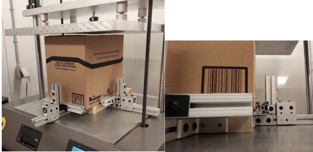
Figure 1. Test setup for box placement with a controllable overhang magnitude.
