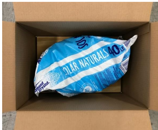
Figure 2. Corrugated container with internal weight
