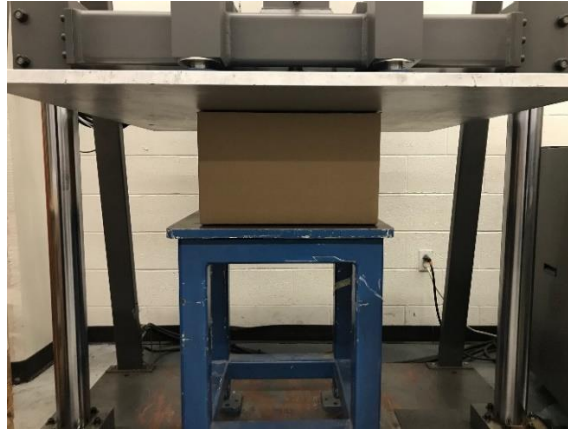
Figure 1. Single box compression test
